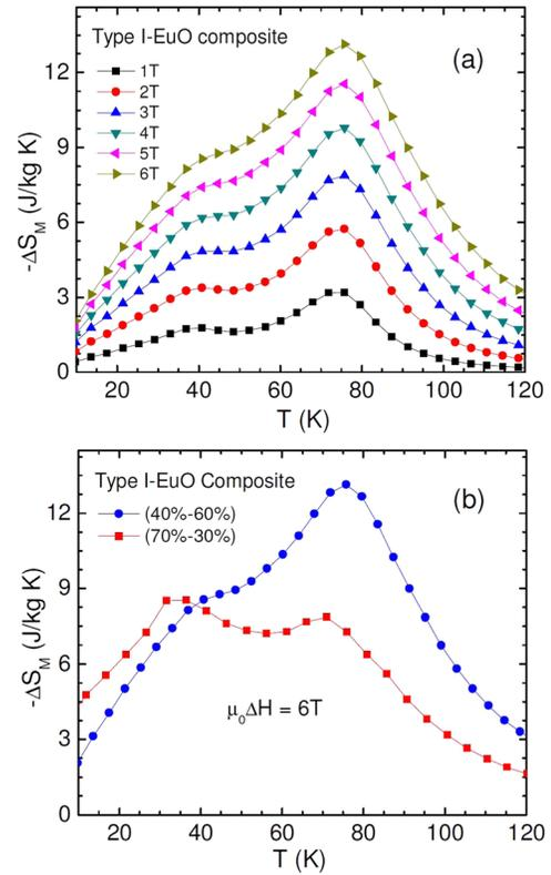
FIG. 2. (Color online) Temperature dependence of  $-\Delta S_M$  at different fields up to 6 T (a) for the 40%-60%  $\text{Eu}_8\text{Ga}_{16}\text{Ge}_{30}$  type-I clathrate–EuO composite and (b) for the 40%-60% and 70%-30% composites.
