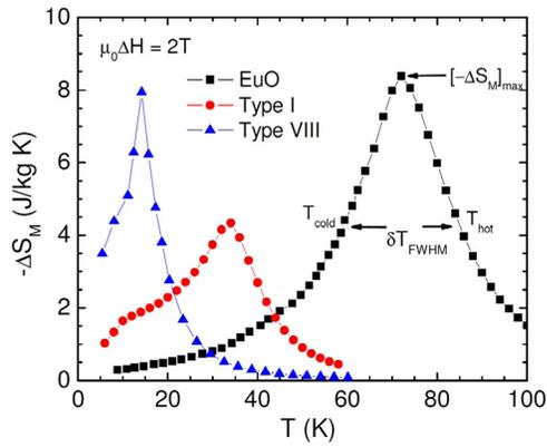
FIG. 1. (Color online) Temperature dependence of  $-\Delta S_M$  at 2 T for the  $\text{Eu}_8\text{Ga}_{16}\text{Ge}_{30}$  type-VIII clathrate, the  $\text{Eu}_8\text{Ga}_{16}\text{Ge}_{30}$  type-I clathrate, and EuO.
